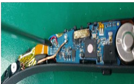
Remove screw (2point).
