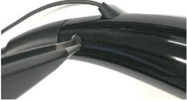
Remove screw cap.
