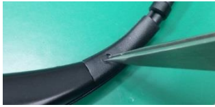
Remove screw cap.
