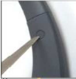
Remove screw cap (2point).
