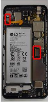
5. Disassemble Connector (2ea) and Main PCB
