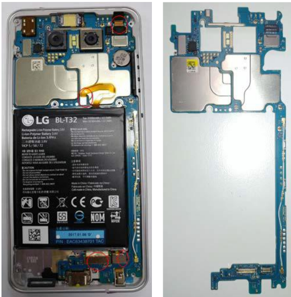
7. Disconnect 4 connectors / main PCB
