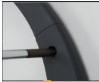
Remove screw (2point).
