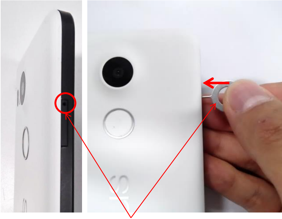
Using SIM ejection, remove SIM tray
