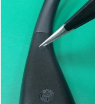
Remove screw cap.
