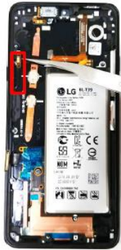
12. Disassemble FPCB PWR Key
