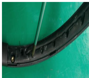
Remove screw (5point).
