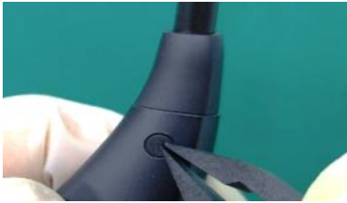
Remove screw cap.
