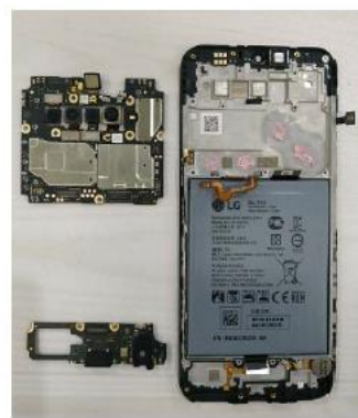
8. Disassemble main PCBA and Sub PCBA
