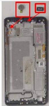
6. Disassemble HW Parts (2ea)
